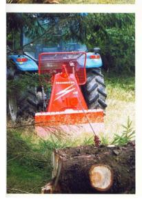
Protective screen guards the tractor in case a cable should brake.
