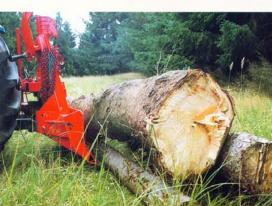
The winch can also be used for log "dozing" and land leveling.
