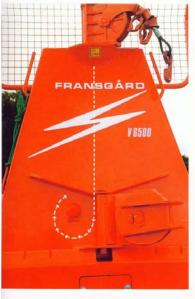
The longer distance between the top pulley and cable drum enables optimal cable spooling.
