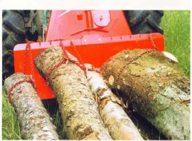
The dozerblade is designed with additional height and a wide log-towing bar to handle even the largest logs.
